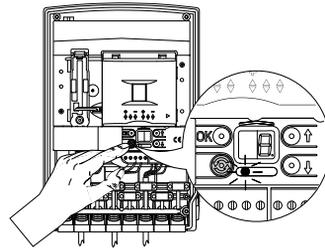
4. Press and hold
