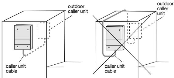
Do not place the products near metal surfaces (screens, fences, gates, etc.) or sources of electromagnetic disturbance:
