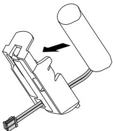
6. Reposition the battery enclosure in the controller.
