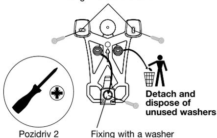
4. Hook the base on to the fixing bracket.
