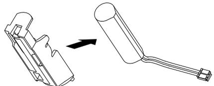
5. Replace it with a new one (ref. 908-21X) making sure to thread the connector through the hole in the enclosure.
