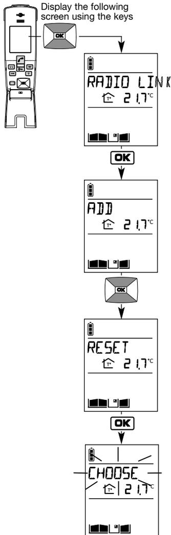
2. Press and hold **OK** until the screen displays OK
