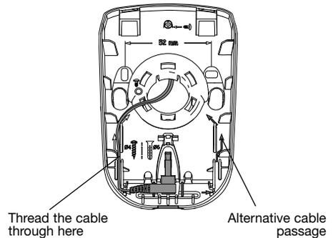
**6.** Thread the power cable into one of the guides at the back of the base.
