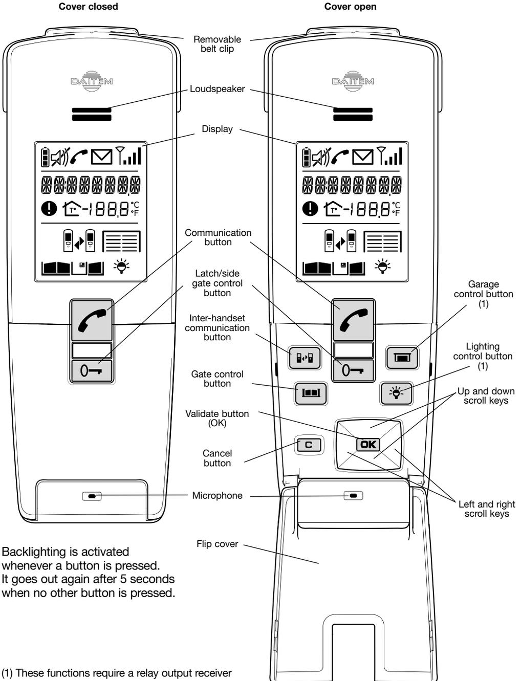
Backlighting is activated whenever a button is pressed. It goes out again after 5 seconds when no other button is pressed.
