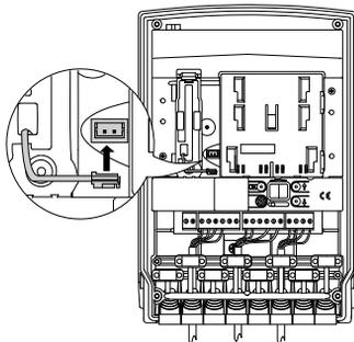
8. Connect a new MPU01X battery.
