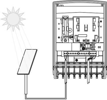
**IMPORTANT: 908-21X battery must be installed for current-based applications. Connect the battery supplied to the connector.**
