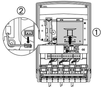
3. Remove the battery enclosure.
