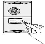
**IMPORTANT:** if you are using an MHF01X or MHF02X translucent outdoor caller unit and a 1-button armoured cover, only the bottom button (KEY 1) is accessible once the cover is in place.
