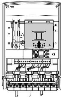
9. When powered, the radio link creation LED lights up red for 2 sec, the outdoor caller unit lights up and also beeps for 2 sec. If this is not the case, check the batteries have been correctly inserted.
