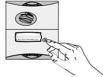
**IMPORTANT:** when using a translucent MHF01X or MHF02X outdoor caller unit and 1-button armoured cover, only the bottom key (KEY 1) can be accessed once the armoured cover has been placed on the unit.
