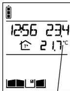
Display of time, indoor and outdoor temperature, gate, side gate or latch status (if position contacts connected).
