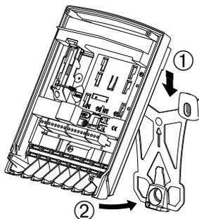
5. Lock the base in place using the locking screw.
