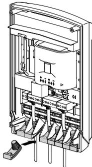
4. Use the cable clamp and screws provided to lock the cables in place.
