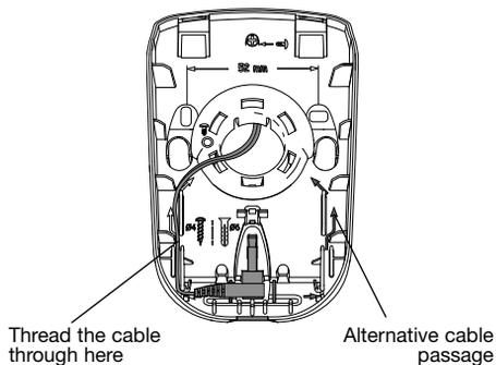
11. Feed the power cable through one of the guides on the back of the base.
