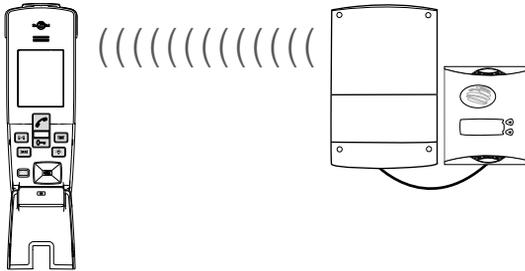
The Light button on the handset controls the lighting connected to the relay output receiver. The handset is considered as the transmitter while the output receiver acts as the receiver.
