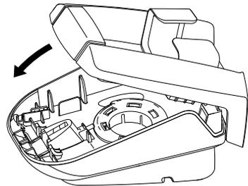
**10.** Tighten the locking screw to prevent the base from being opened by mistake.
