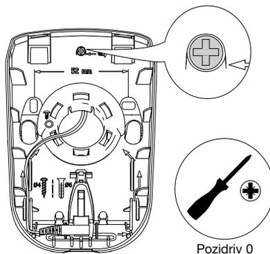
8. Rotate the back of the base until it is in wall position.
