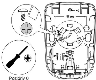
7. Insert the screw here and tighten it.
