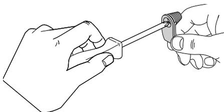
2. Cut the cables to the necessary length and then thread them through the grommets. Expose the end of the wires over a length of approximately 1 cm.
