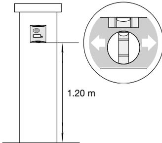
2. Mark and drill the outdoor caller unit holes with a  $\varnothing$  6 mm drill bit. Also mark the place where the cable feed hole has to be drilled ( $\varnothing$  8 mm min. recommended).
