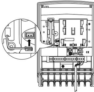
then connect the battery by positioning it on the rails and sliding it downwards.
