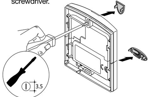
5. Thread the cable through the hole knocked out in step 3 and screw the caller unit in place. Put the screw covers back.
