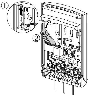
4. Remove the flat battery from its box.
