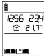
Display of time, indoor and outdoor temperature, gate, side gate and latch status (if position contacts connected).
